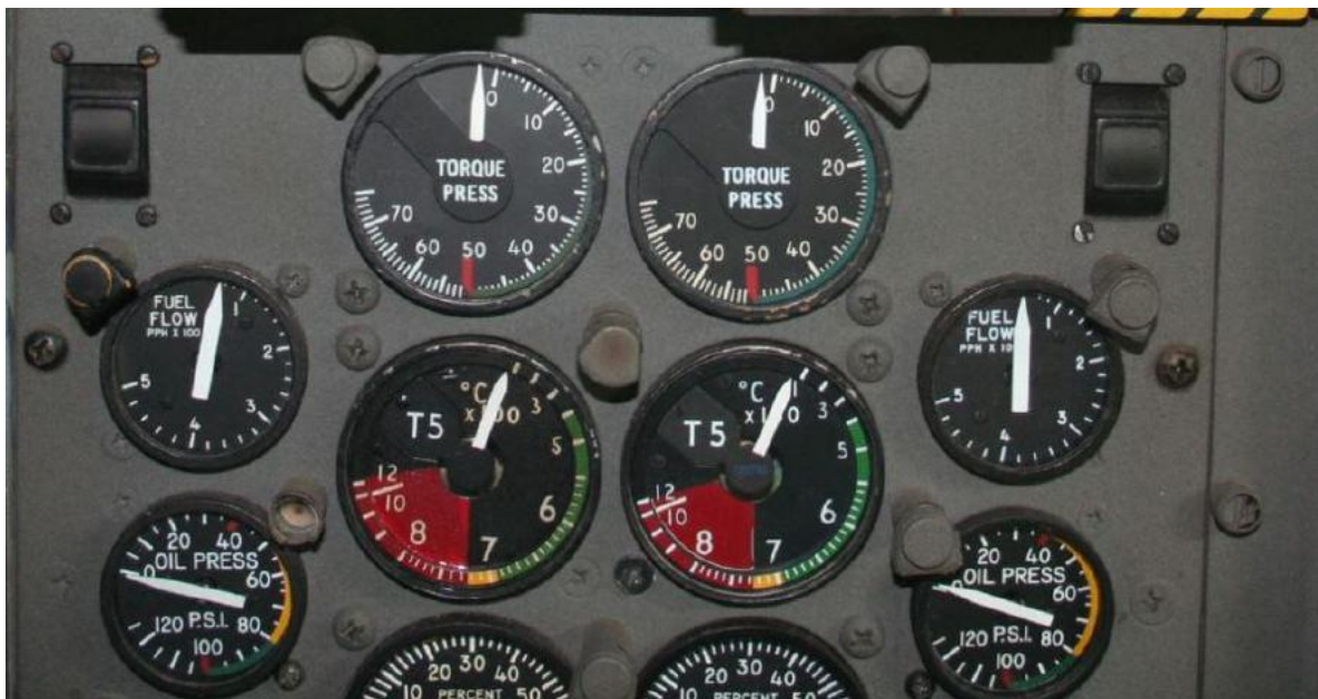
Oil Pressure and T5 Gauge
